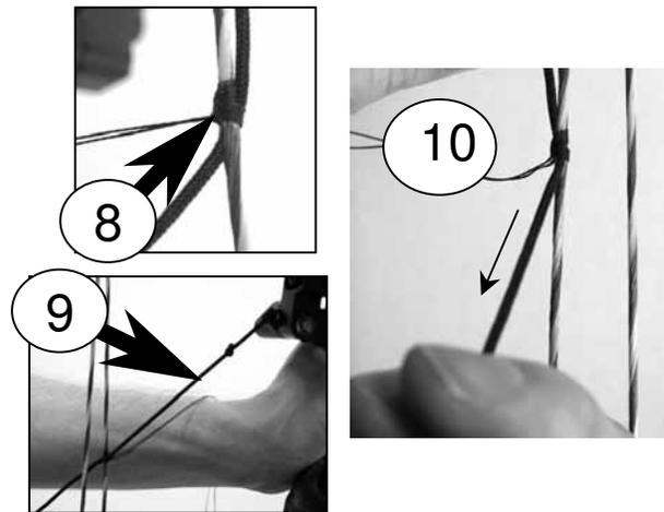
11. Continue the serving over the cable and rope until the serving is about an inch long.
