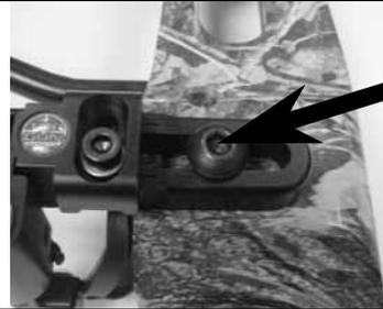
4. Adjust the center shot using adjustment screw "A". Adjust the elevation by using screw "B". Note that there are two threaded holes in each location to allow for greater adjustment.
