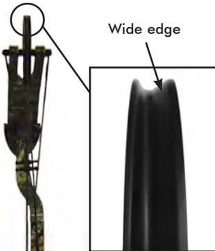
Some PSE bows are equipped with a special asymmetric idler wheel, which is assembled on the top limb. It is essential that the idler be oriented properly. The wide edge of the idler always goes to the cable guard side of the bow. The illustration shows the proper orientation of the idler for a right-handed bow when viewed while holding the bow as it is shot.
