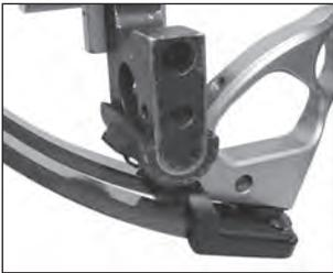
Back the limb bolts out 4 turns from the bottom setting and position the pressure points on the riser as close to the limbs as possible **WITHOUT** making contact with the limbs as shown in the photo. The pressure points must not contact the limbs at any time during servicing.
