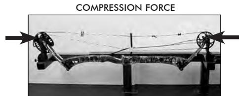
Compress ONLY far enough to loosen the string and cables. Over compressing could break the limbs and cause personal injury. Any damages incurred from over-compressing will not be covered under warranty.
