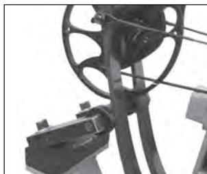
Service such as peep and vibration damper installation and string replacement can be performed with a Pocket Press portable bow press (item #01169) available from your local PSE dealer. Item #01170 and #01031 are pocket presses also available for alternate axle-to-axle lengths.
